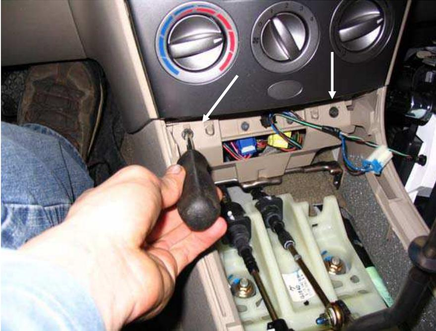
**Now remove the 4x12mm bolts located at each corner of the shifter cage. Raise the cage up to clear the studs. Pry the steel sleeves up and out of the rubber grommets. Now push the rubber grommets out through the bottom.**
