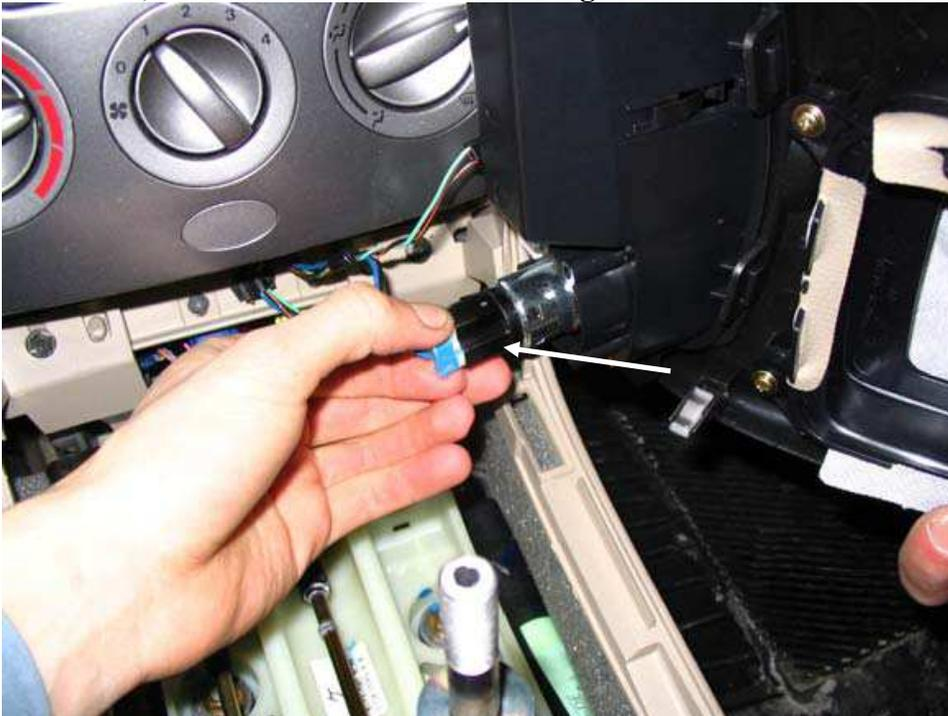
**-Disconnect the wire located behind the handbrake. You will need the needle nose pliers to detach the wire from the console. Depress the plastic tabs and push down. Now disconnect the plug by pushing on the tab and pulling it off.**
