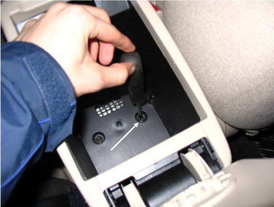
**-Now disconnect the wires for the cigarette lighter. Push the tab and disconnect it. The other plug next to it just needs to be pulled while pressing the small tabs on either side, but be careful with it as it's a light bulb.**
