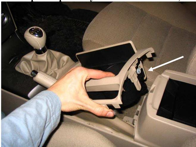
**-Locate the plastic caps on each side of the center console in front of the front seats. Carefully remove them by gently inserting a little flat screw driver and prying the cap off. Remove the screws with the appropriate screw driver.**
