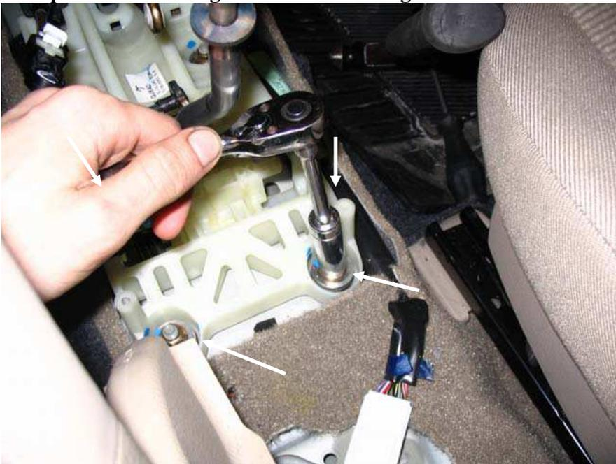
**-Install the JBR Shifter Bushings on to the studs. Place the shifter cage back over the studs indexing the cage with the small diameter side (up) of the bushings.**
