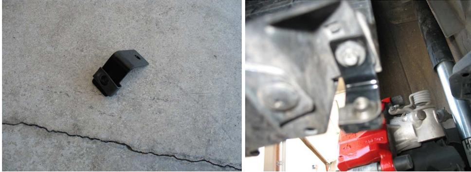
5. Place 2 edge clips over the 2 holes of the inner fender liner where the rivets or used to be. Place 2 black nylon washers on 2 short stainless bolts and 1 washer over 1 long stainless bolt. Place the inner fender liner back behind the lip of the rear bumper and center the edge clips using a philips head screw driver or punch.
