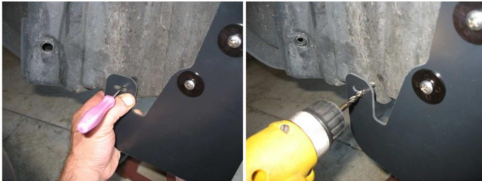
8. Place the long bolt and washer through the 4<sup>th</sup> mounting hole. Place 1 black nylon spacer behind the mud flap and in front of the fender liner, then push the bolt through the fender liner. Secure the bolt using 1 stainless flat washer first, then 1 stainless lock washer and 1 stainless nut. Tighten the bolt using a philips head screw driver and a wrench from behind the fender liner. Re-install 3 of the 6 inner fender liner fasteners previously removed in step 2.
