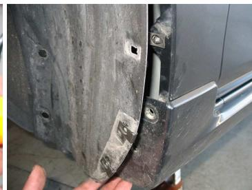
3. Place 2 edge clips over the lowest two holes of the fender liner and one on the tab of the fender.
