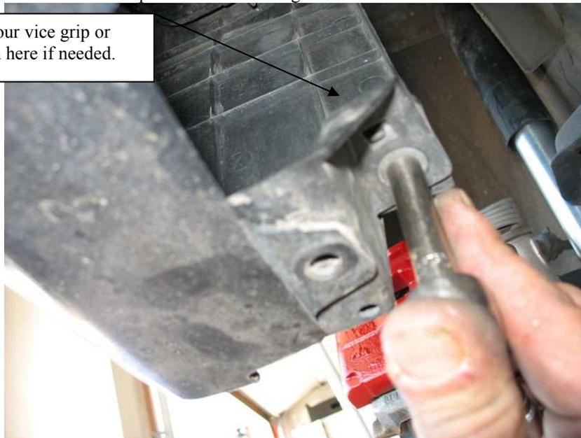
4. Assemble 1 angle bracket with 1 edge clip. Place the edge clip on the slotted side of the angle bracket with the angle bracket facing the front of the vehicle and the thread side of the edge clip on the rear side of the angle bracket. Install the angle bracket and edge clip assembly using the bolt removed in the previous step.
