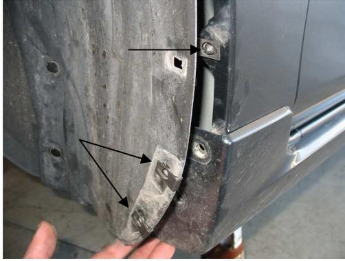
4. Re-install the liner as it was prior to removal. The clips may move during the installation of the liner. To center them use a philips head screw driver or punch.
