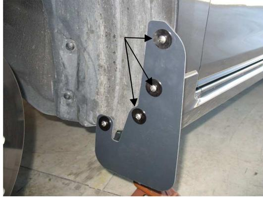
7. Use a scribe or sharp punch to pierce the inner fender liner in the center of the 4<sup>th</sup> mounting hole. Then use the drill & 1/4" drill bit to drill a hole in the inner fender liner.
