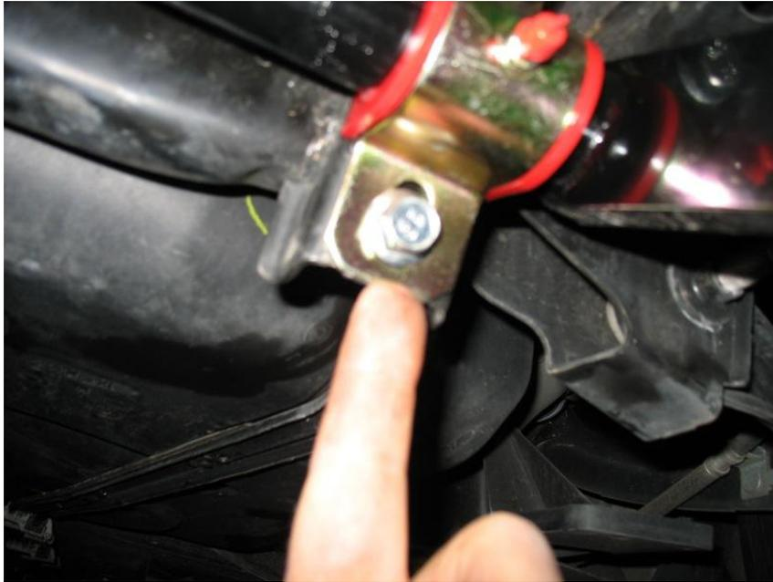
10. Place 1 lock washer on each end link and tighten the 2-17mm nuts removed earlier using a 17mm closed end wrench and a 5mm allen wrench.
