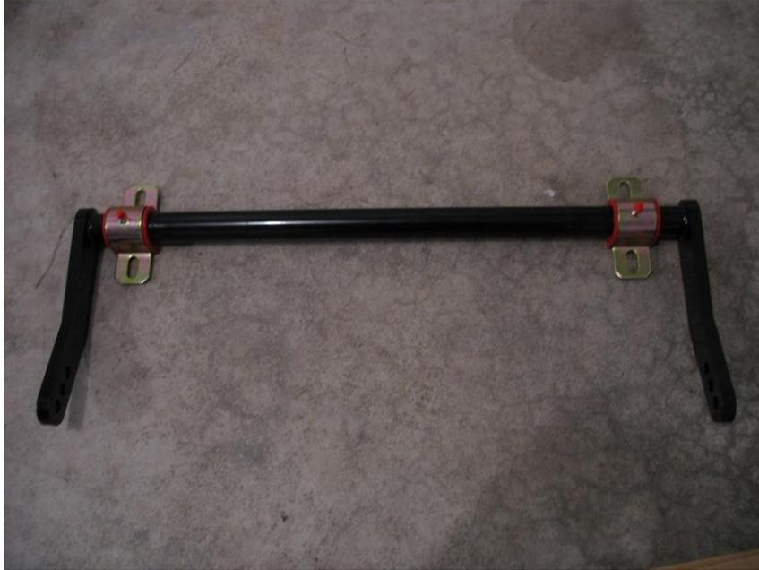
6. To install the new JBR Sway Bar in to the vehicle first by placing both of the end links in to the desired hole in the end of the sway bar arm. The recommend staring point is the center hole. The hole closest to the front of the vehicle is the stiffest setting. The hole closest to the rear of the vehicle is the softest setting.
