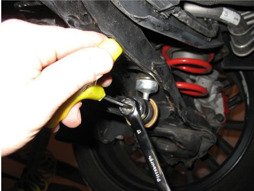
4. Remove the 4-14mm bolts securing the end link brackets and bushings to the vehicles sub-frame. Then remove the factory sway bar from the vehicle.
