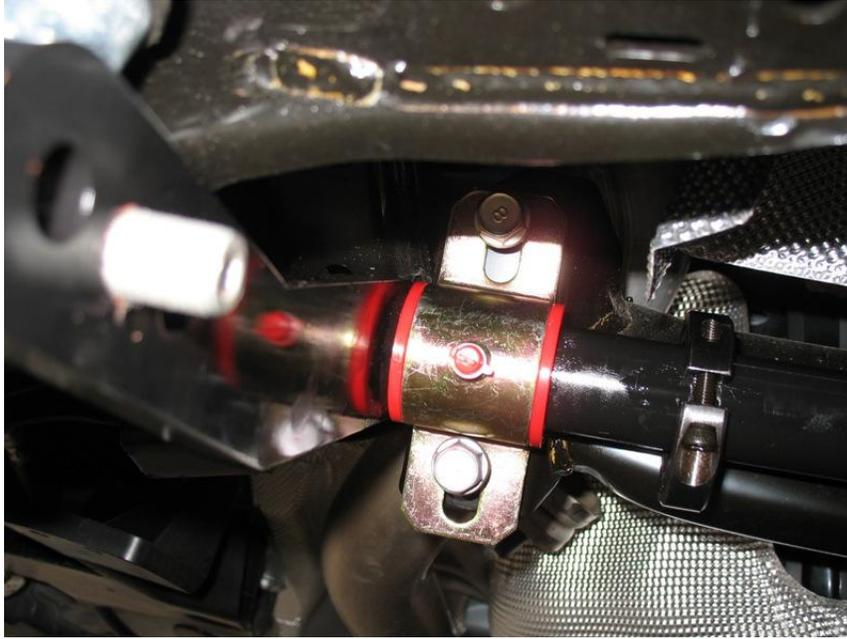
8. Center the sway bar by sliding it left or right and ensure the gap between the arms and the outside edge of the bushings are equal.
