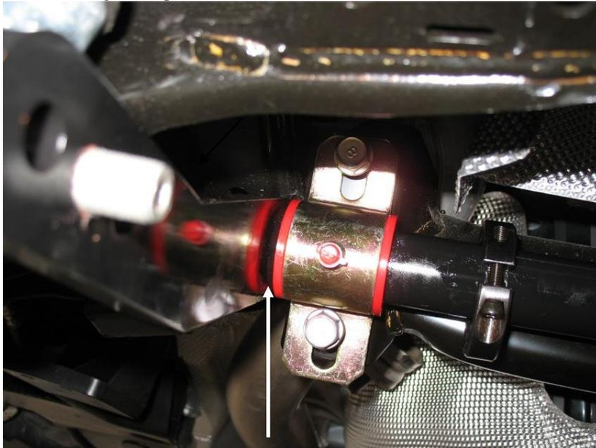
9. Raise and torque the 4-14mm bolts to 30-35ft/lbs so the bolts are centered in the brackets.
