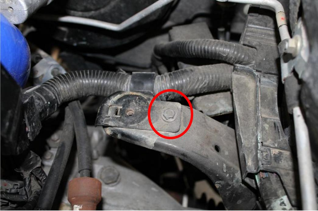
7. Place 1 flat washer on to each of the 3 included button head screws and using a 4mm Allen Wrench install your new JBR 51R battery tray in to the vehicle.
