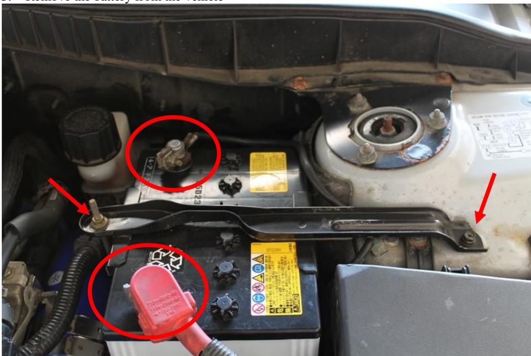
4. Unclip the strap securing the wire loom to the front of the battery tray.
