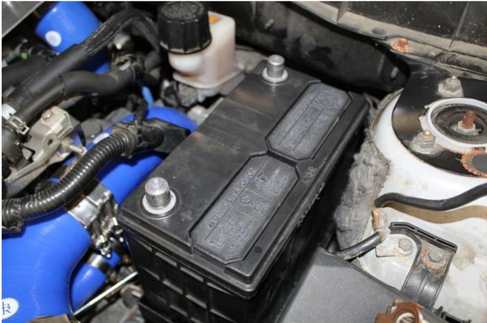
9. Raise the J-hooks and slide the hold down strap over them. Place 1 flat washer on to each J-hook then a lock nut and tighten.
