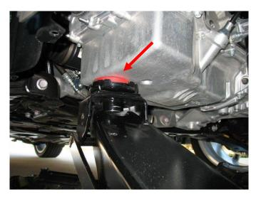
3. Now, remove the two 17mm nuts securing the top potion of the factory mount to the motor. Also remove the 14mm nut securing the rear portion of the mount to the inner fender and the front 14mm bolt securing the base of the mount to the frame. Next, remove the rear 14mm bolt (Not Shown) securing the mount to the frame.
