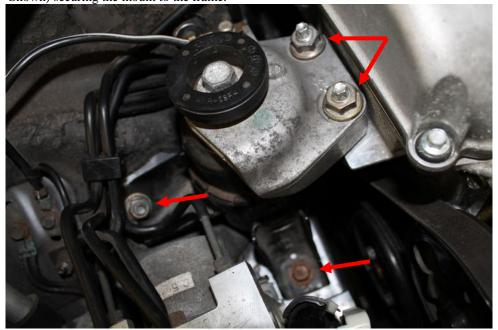
4. Now remove the 10 mm bolt securing the ground strap to the top of the mount.
