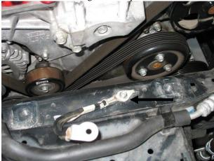
7. Bend the end of the ground strap previously bolted to the mount on a 45\* angle.
