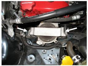
6. Remove 1x 10mm bolt and remove the ground strap.
