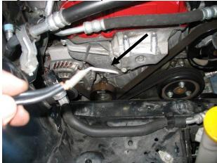
8. Flatten the tab on the end of the ground strap previously bolted to the chassis.
