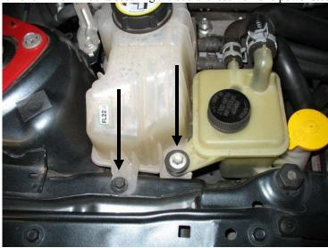
4. (All Years) Remove the coolant and power steering reservoirs by inserting a flat head screw driver in to the tabs and pulling up.
