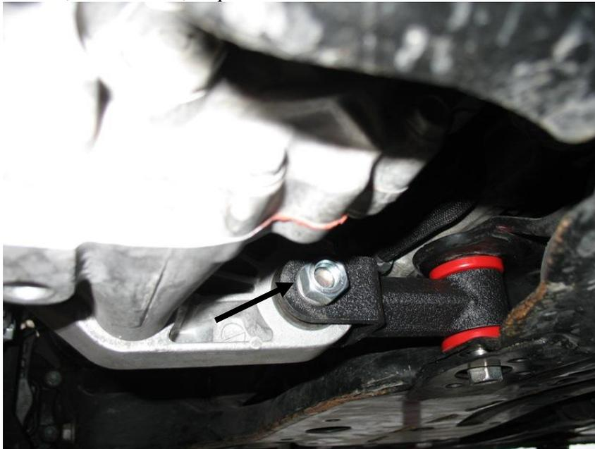
7. Tighten and torque the bushing bolt to 70 foot-pounds using a 17mm socket, socket wrench, and torque wrench.
