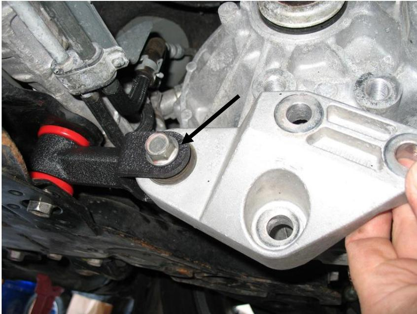
5. Pivot the transmission bracket up in to place and install the 3 bolts previously removed. Rocking of the engine may be required to align the bolts. Using a 19mm socket, socket wrench and torque wrench tighten and torque the bolts to 70 foot-pounds.
