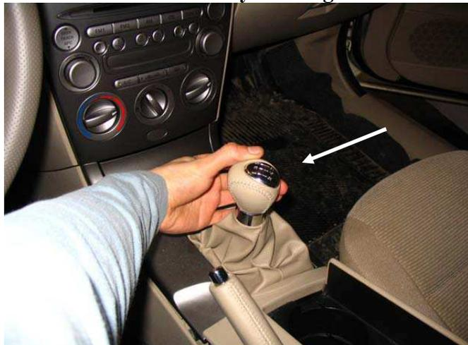
**- Hold the inside edge of the console around the shift boot and grab the cup holder beside the handbrake and gently pull on it until it unclips. Don't try to get the two parts apart or you could break them, remove them together.**
