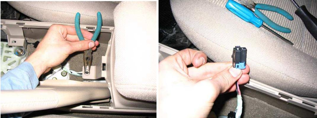
**-Remove the 2 screws located on either side of the console just in front of the emergency brake.**
