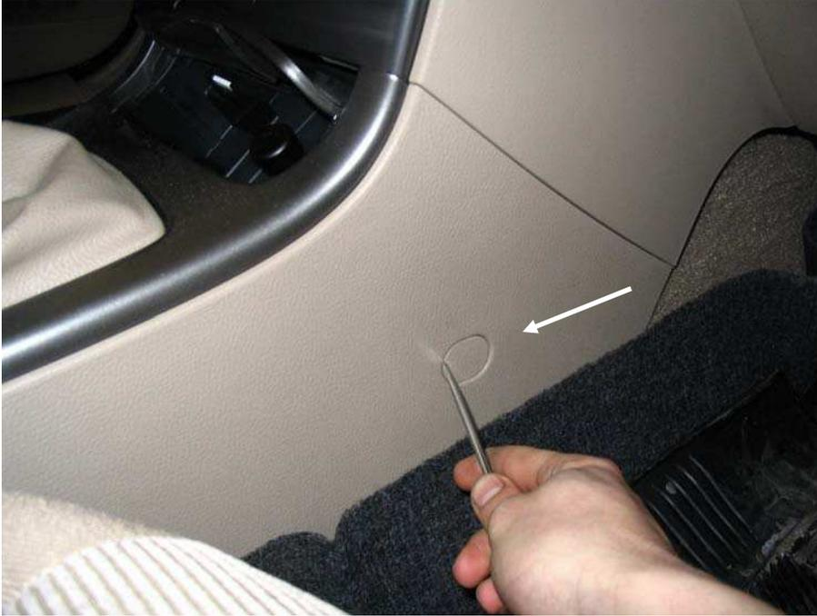
**-Move the front seats fully forward. Remove the plastics caps and screws like those in the front. Careful during reassembly, the caps only fit one way; one tab is bigger than the other, so don't force them.**
