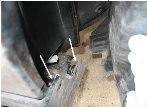
5. Place 1 edge clip over the remaining metal tab in the fender.
