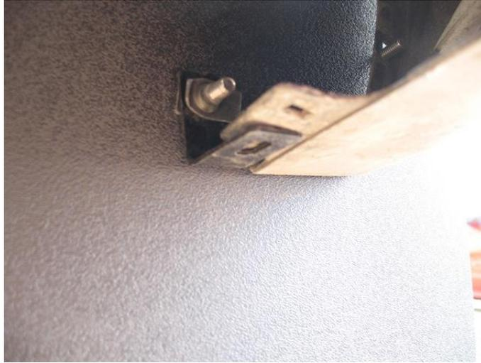
11. Re-install the last fastener from the fender liner through the angle bracket and tighten to the bottom rear of the bumper.
