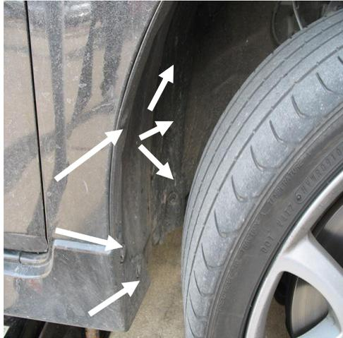
3. Pull the fender liner out from behind and away from the fender.
