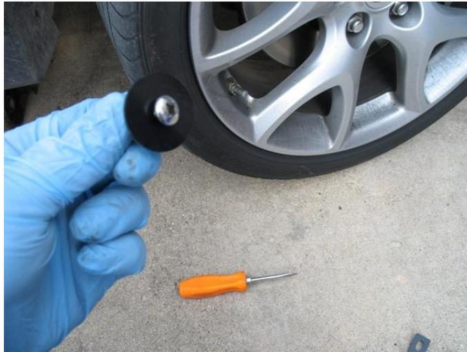
8. Install the front right mud flap with the textured side facing the rear of the vehicle using the 3 bolts and washers. Then secure the mud flap to the fender. Re-install the 3 inner most fasteners for the fender liner.
