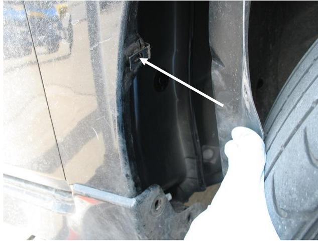
6. Re-install the fender liner as it was prior to removal . The clips may move during the installation of the liner. To center them us a philips head screw driver or pick.
