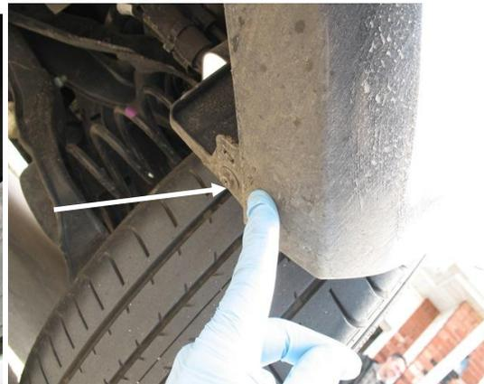
3. *Carefully* trim off the notches in the fender liner using a sharp razor knife or razor blade.
