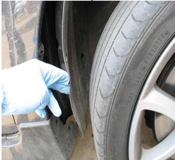
4. Place 2 edge clips over the lowest two holes of the metal portion of the fender.
