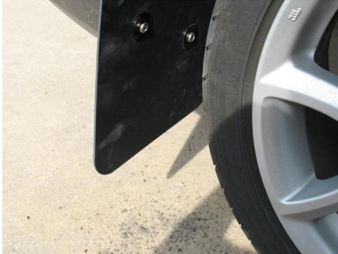
9. From below and behind the bumper place 1 flat washer, 1 lock washer and 1 nut on each of the bolts. Then secure the mud flap to the fender ensuring the mud flap is plum and level to the side of the vehicle and the ground then tighten.
