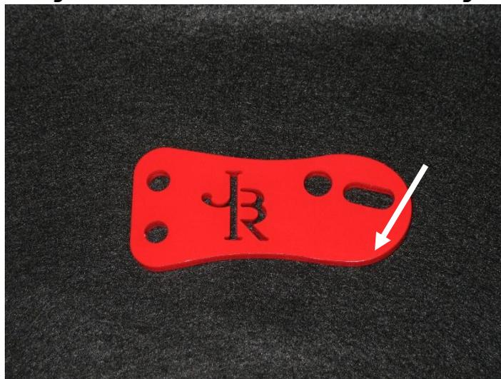
Attach by applying one drop of the supplied Loctite, lock washer and nut. Tighten as shown using 2 13mm wrenches.
