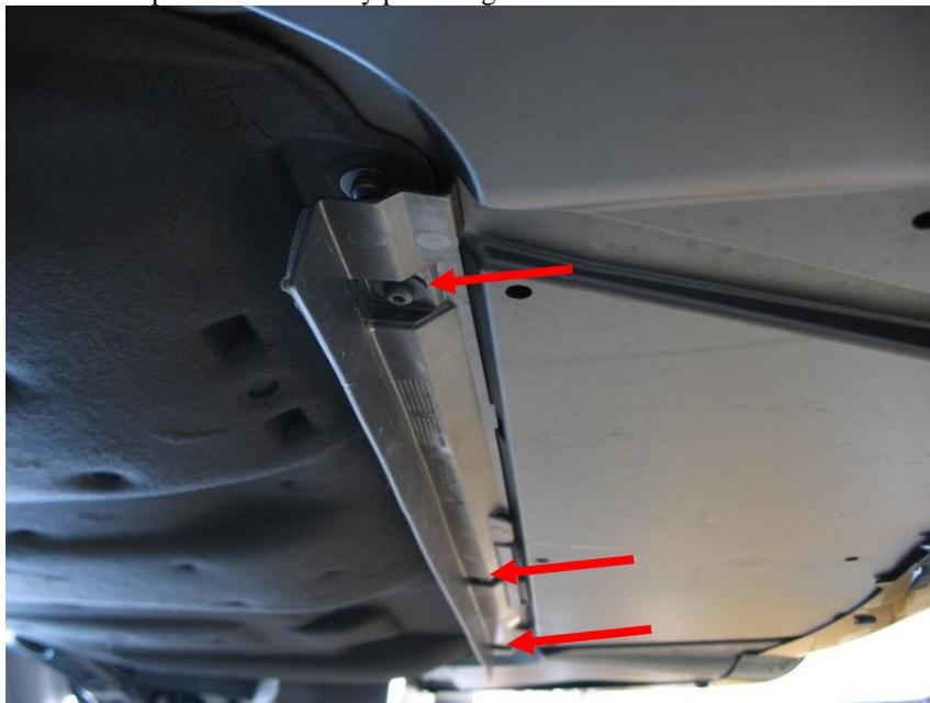
2. Remove the remainder of the belly pan use the T-30 torx bit..
