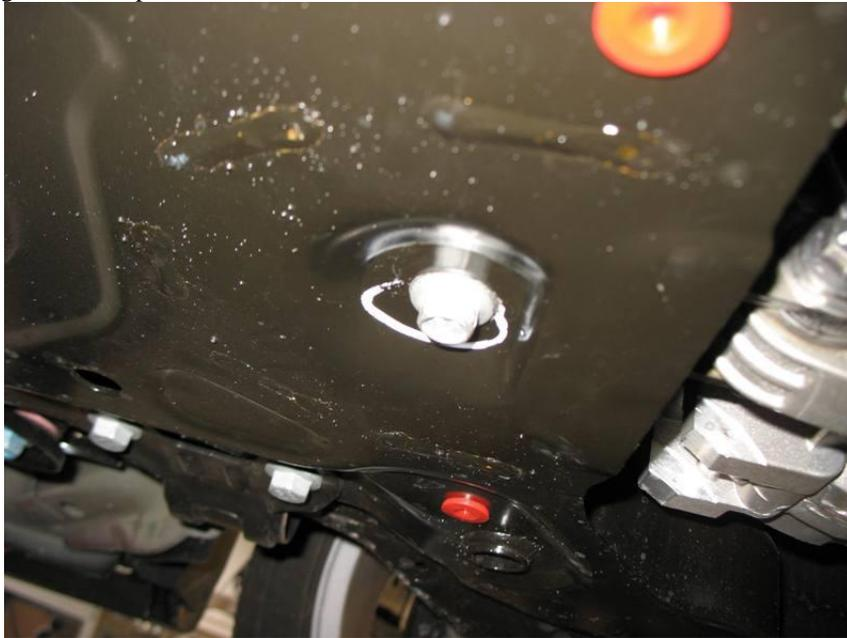
7. Push the OEM mount towards the rear of the vehicle deep in to the sub-frame then with a 15mm closed end wrench remove the 2 bolts shown below that secure the motor mount bracket to the transmission. The motor may need to be pivoted towards the front to remove the rear most bolt. The engine pivots easily by hand.
