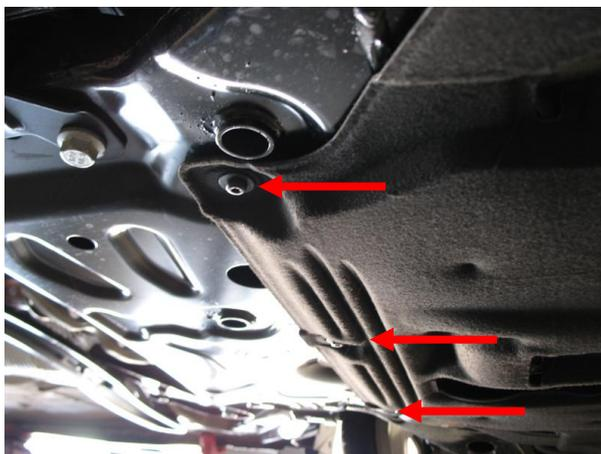
3. Once the belly pan is removed and the rear mount is exposed, remove the 6 nuts shown below that secure the down pipe support bracket to the transmission with a 13mm 6-point socket and 6" extension.
