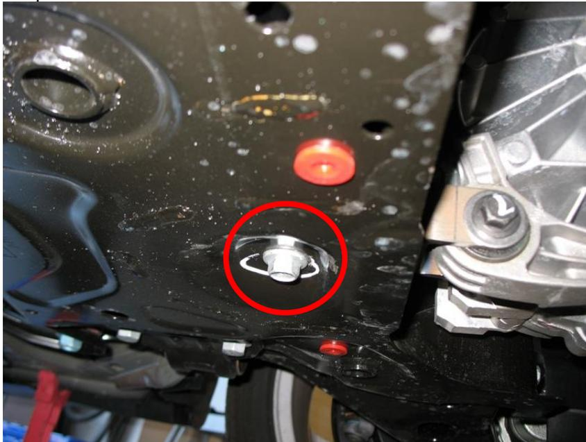
12. Reinstall the downpipe support bracket, tighten all 6 nuts and reinstall the belly pan.
