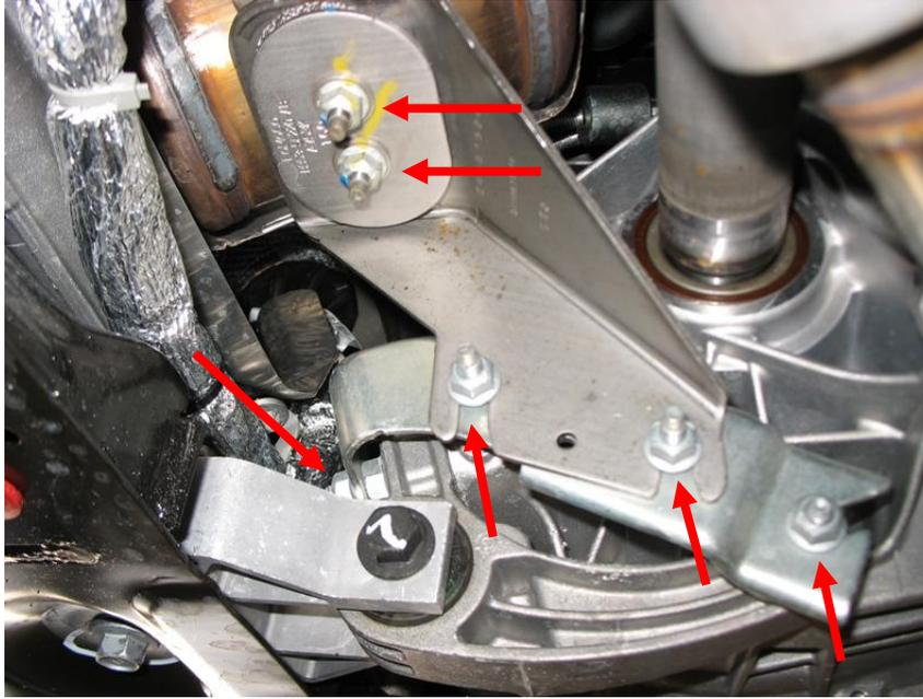
4. With the 6 nuts removed in the previous step now, remove the bracket that secures the down pipe to the transmission by applying pressure to the bracket and pushing it towards the passenger side of the vehicle.
